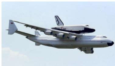
Giant plane An-225 produced by Kiev mechanical plant is transporting the space shuttle “Buran”
