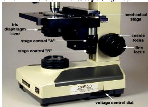
Fig. 18. Focusing of microscope: iris diaphragm lever: moving the lever to the left increases the light; moving the lever to the right decreases the light; stage control "A": moves the mechanical stage holding the slide forward and backward; stage control "B": moves the mechanical stage holding the slide left and right; coarse focus: turning the knob away from you raises the stage; turning the knob towards you lowers the stage; fine focus: turning the knob away from you raises the stage; turning the knob towards you lowers the stage.
