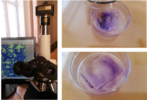
Fig. 4. Getting of microorganisms biofilms on a glass
