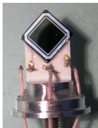
Fig. 4. The base unit with mounted detector of 5×5 mm (view on the front side of detector)
