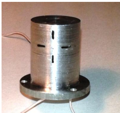
Fig. 5. A sealed module for detection of thermal neutrons on the basis of uncooled PSD ( 5 \times 5 mm) and a metal gadolinium converter in an aluminum housing
